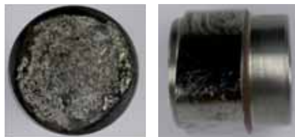
Engine wear that can result from incorrect wintering procedure.
