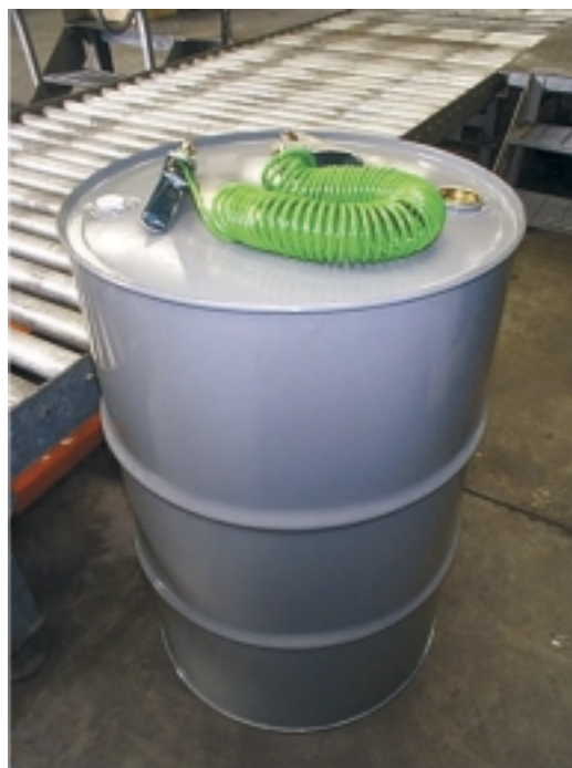
Typical portable grounding cable for drums
