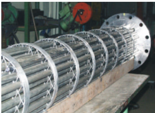
Bundle of an EMbaffle heat exchanger
